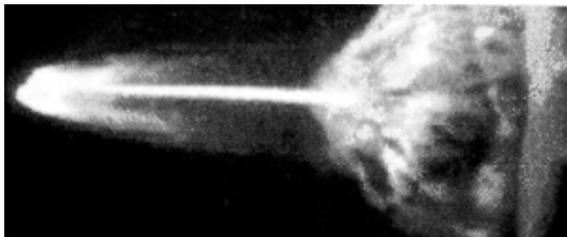
Fig. 6. Shaped charge jet 40 mks after detonation [22].
