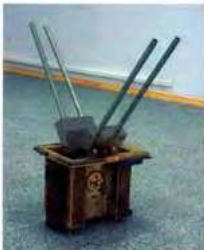
Fig. 2. Plasma dielectric antenna with four jet [8].
