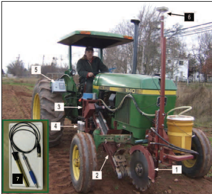
Fig. 3. Soil nitrate mapping system with six sub-units: (1) soil sampler, (2) soil metering and conveying, (3) nitrate extraction and measurement, (4) auto-calibration, (5) control and (6) global positioning system, with (7) inset showing Orion 97-07 ionplus \text{NO}_3^- -ISE used for measuring soil nitrate (adapted from Sibley, 2008).
