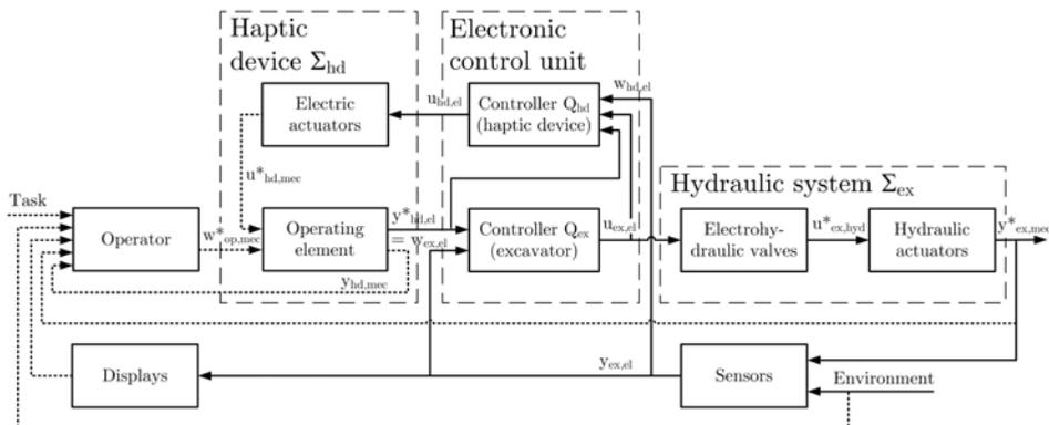
Fig. 6. Haptic human-machine interface of an excavator
