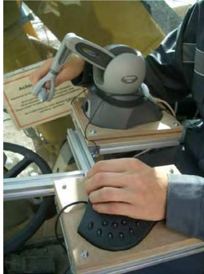
Fig. 5. Test excavator equipped with operating devices
