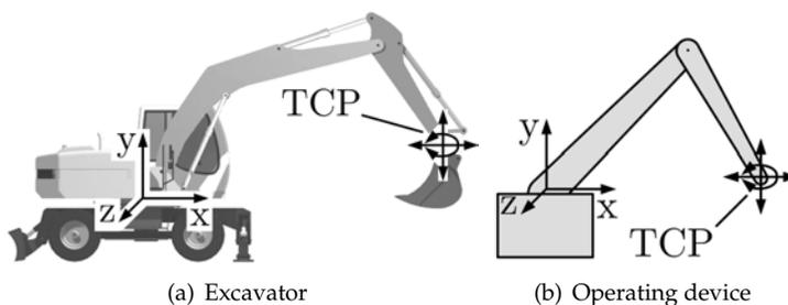
Fig. 1. Operating device resembles the manipulator geometry
