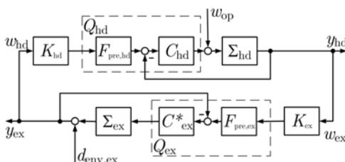
Fig. 7. Master-slave control loop
