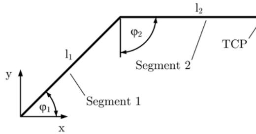
Fig. 10. Kinematics of a SensAble Phantom Omni
