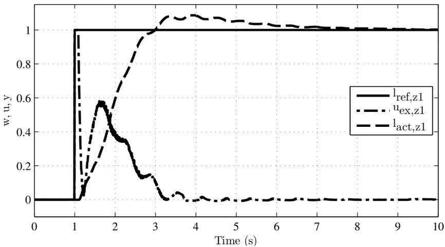
Fig. 15. Step response of the excavator’s boom cylinder
