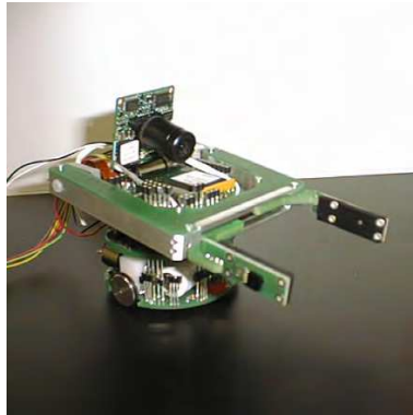
Fig. 2. Khepera robot equipped with a color CCD camera and a gripper.
