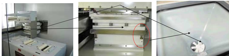
Fig. 2. Metallic contamination on Wet process tool, EDX identification
