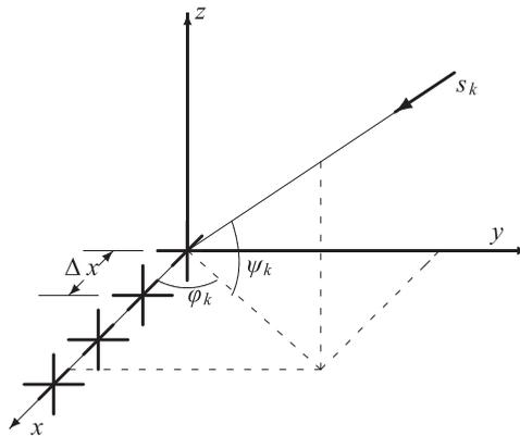
Fig. 1. 2D-DOA on a vector-sensor array
