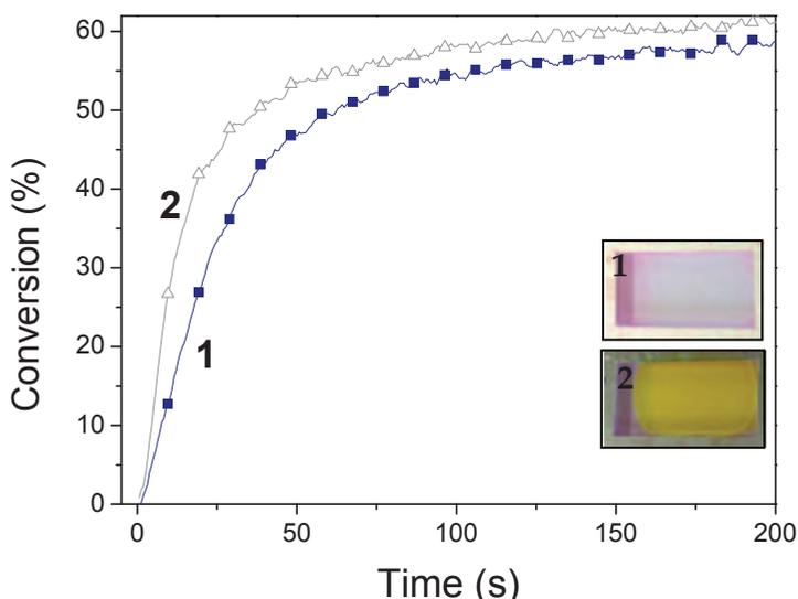
Fig. 4. Real-time FTIR kinetics conversion curves of the acrylate double bonds for visible curing at 532 nm: (1)  $\text{EO}^{2-}$ / MDEA, 0.1 wt % / 3 wt % and (2)  $\text{EO}^{2-}$ / MDEA /  $\text{AgNO}_3$ , 0.1 wt % / 3 wt % / 1 wt %. Inset: View of 30  $\mu\text{m}$  thick samples (1) and (2) after curing.
