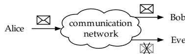
Fig. 1. Communication system with a transmitter (Alice), a legitimate receiver (Bob) and an eavesdropper (Eve).
