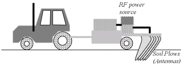
Fig. 15. Schematic for a Portable RF-Soil processing system.
