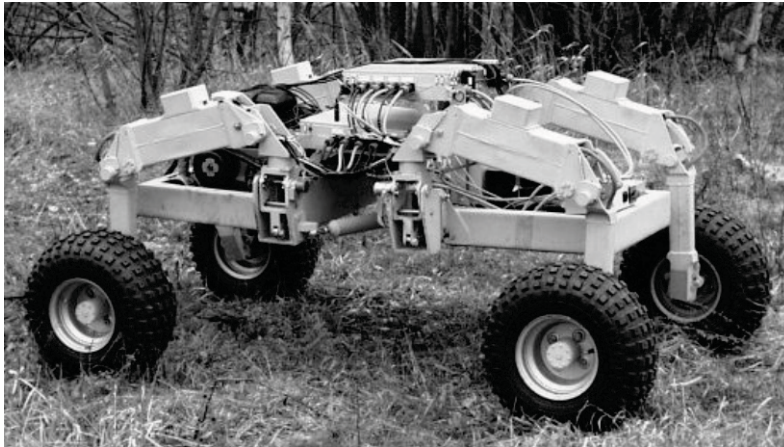
Fig. 4. WorkPartner in an early stage of development, where the structure of the legs and front and rear bodies can be seen.
