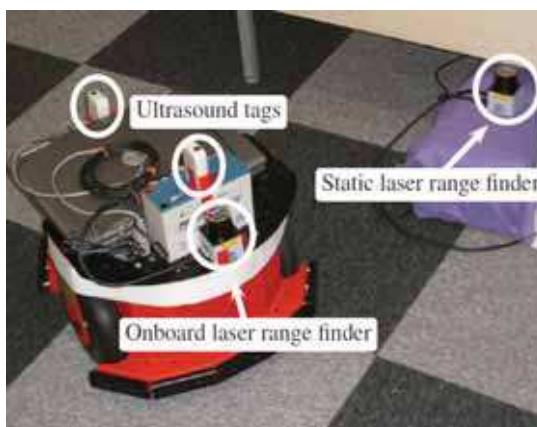
Fig. 5. Experimental setup: the mobile robot and one of the distributed laser range finders.
