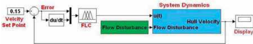
Fig. 10. Closed-loop system using stand-alone FLC used in simulation.
