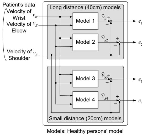
Fig. 13. Block diagram of quantitative evaluation method
