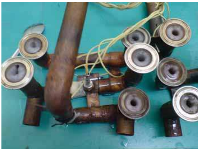
Fig. 5. Ice layer formed in the detached CC
