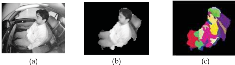
Fig. 8. Preliminary segmentation results for adult occupant, (a) adult image, (b) preliminary segmented adult, and (c) region labeled adult image (Farmer & Jain, 2005).
