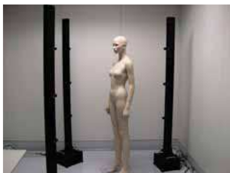
Fig. 8. Human body measurement system.
