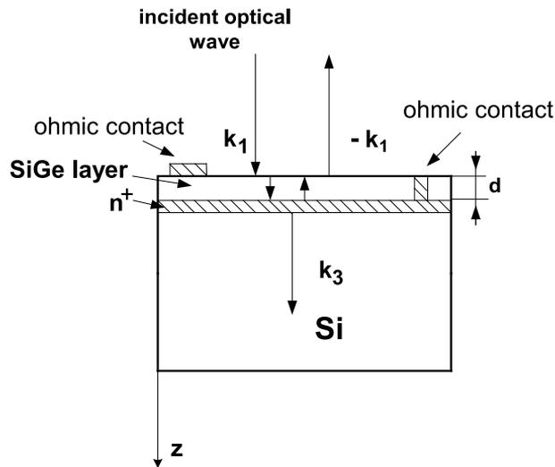
Fig. 4. Illuminated SiGe layer on a Si substrate
