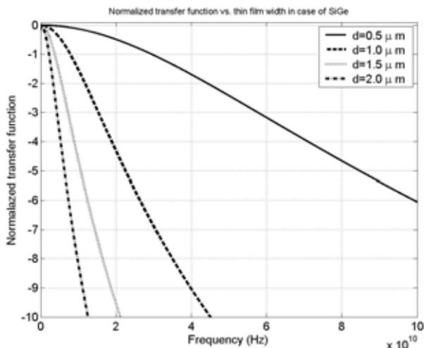
Fig. 5. Normalized transfer function  $|\overline{N}_1(\omega)|$  for different SiGe layer thicknesses  $d = 0.5; 1; 1.5; 2\mu m$
