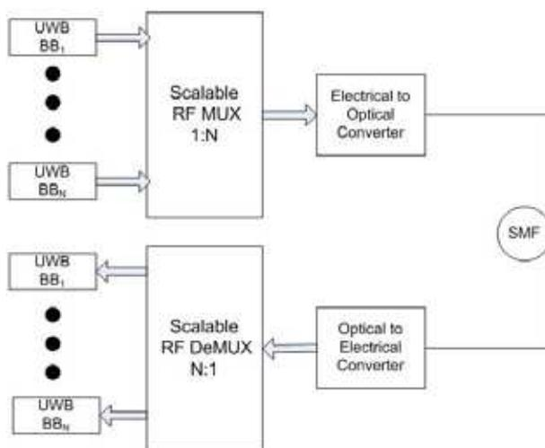
Fig. 1. 61.44Gb/s based on parallel RF/serial optics with  $N = 128$  channels
