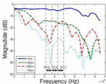
Fig. 12. The measurement results for the optical link frequency response
