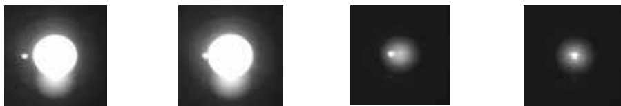
Fig. 7. Offset launch of a restricted spot into a fibre core. From left to right, this injection spot is going from outside the core up to its centre.
