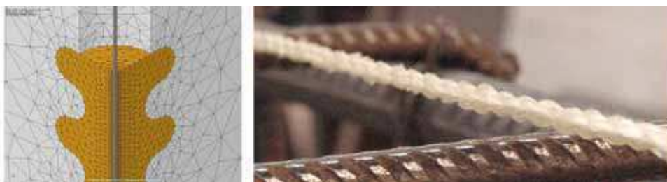
Fig. 13. Sensor coating. On the left, FEM figure of the sensor developed at LCPC; On the right, the sensor actually made by the IDIL company from the theoretical model.
