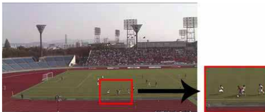
Fig. 1. Clipping from the HD image to a SD image using digital camera work
