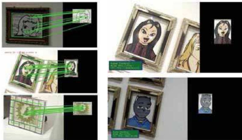
Fig. 20. Real museum test: (left) with image correspondences and recovered pose displayed under various lightings and viewpoints, and (right) with retrieved information displayed.
