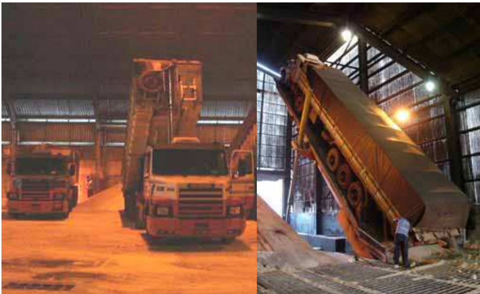
Fig. 2. Most common types of truck: a) Dump truck; b) Bulk truck tipped by a hydraulic tipping bridge.
