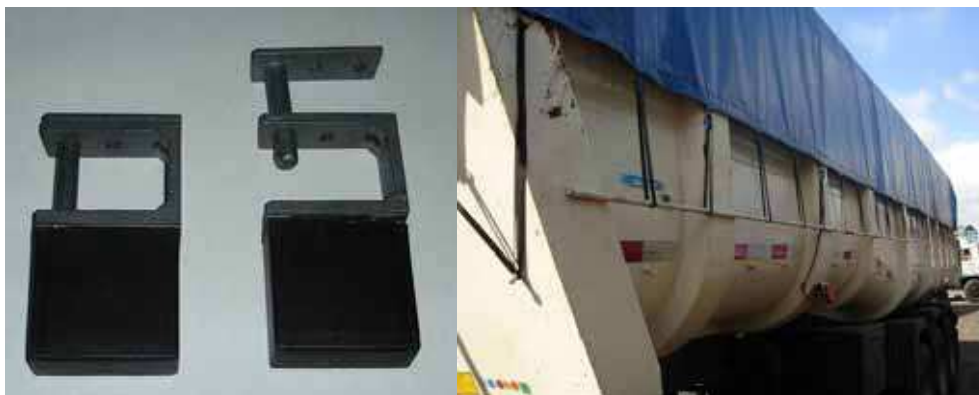
Fig. 7. a) Padlock tag assembled, opened and closed; b) One type of trailer showing the iron bar where the padlock tag is attached.
