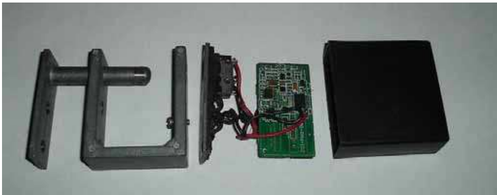
Fig. 6. Active tag in a padlock shape with opening detector disassembled.
