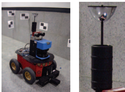
Figure 1. Pioneer P3-AT robot and Catadioptric system that provides omnidirectional images
