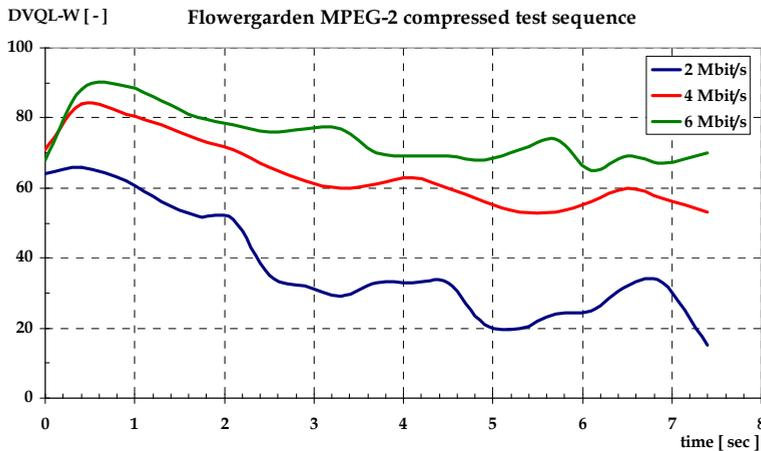
Fig. 10. Video image quality analysis of the „Flowergarden“ test sequence. The DVQL-W metric and according quality varies with the MPEG-2 compressed test sequence bitrate.
