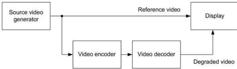
Fig. 3. General arrangement for the DSCQS method evaluation
