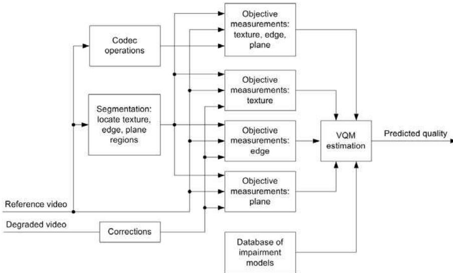
Fig. 6. Simplified block diagram of the IES metric
