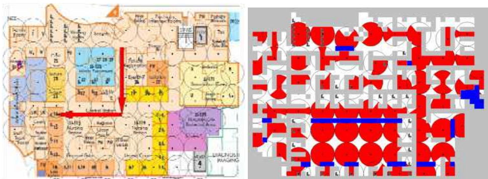
Fig 10. Trajectory of outlier patient with high temporal and spatial error (left), reader coverage (right), interference regions in blue, readable areas in red
