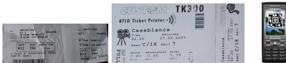
Fig. 5. Boarding Pass with bar code, and with RFID in a paper, 2D bar code in a mobile phone
