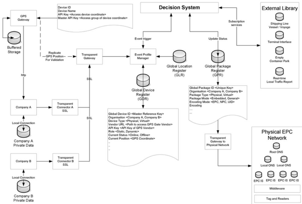
Fig. 8. Overall Design of the transparent virtual framework
