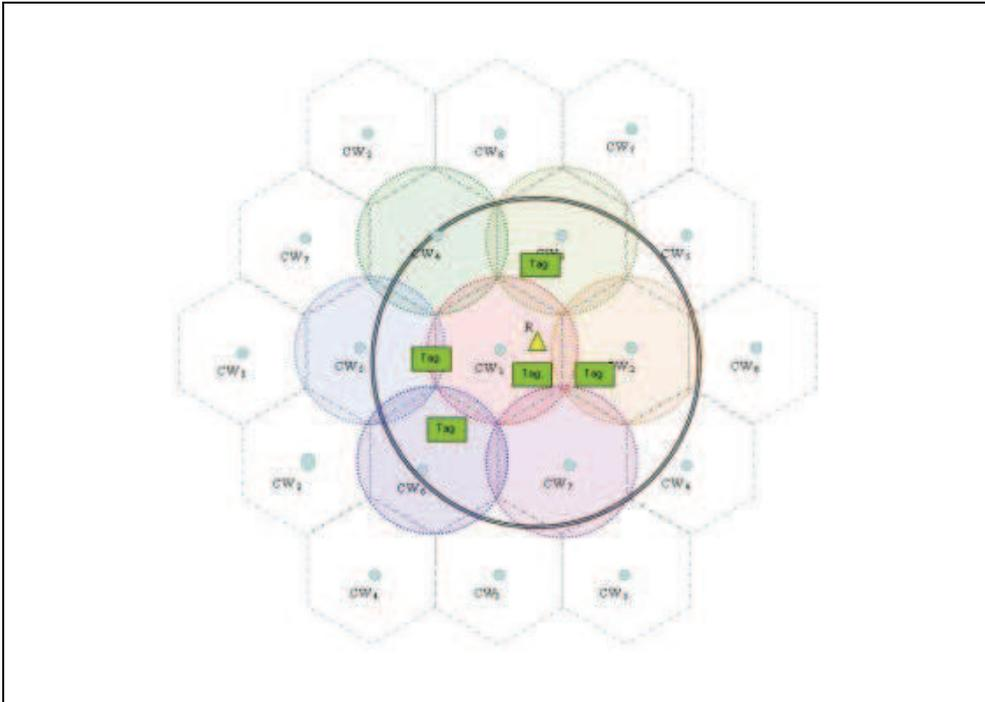
Fig. 2. A possible deployment of a multi-carrier RFID system, where R denotes the reader and  $CW_i$  denotes that the CW using the  $i$ -th frequency band.
