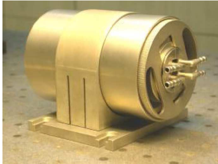
Faraday isolator with slab magneto-optical elements
