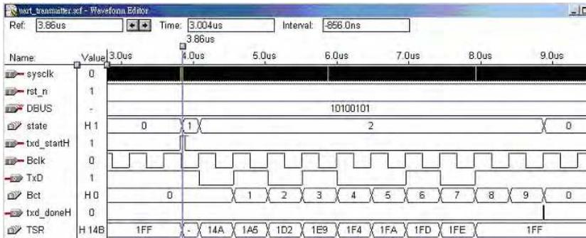
Fig. 10. UART transmitter transmitting 0xa5.
