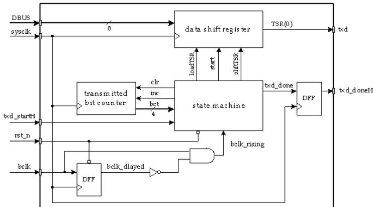
Fig. 8. Functional block-diagram of the UART transmitter.
