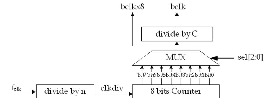
Fig. 2. Architecture of the baud rate generator.
