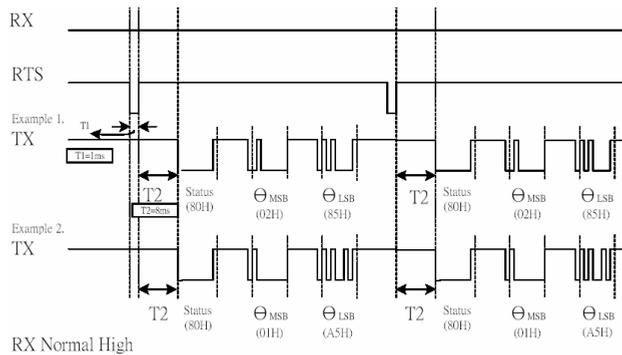
Fig. 12. Timing chart of normal mode.
