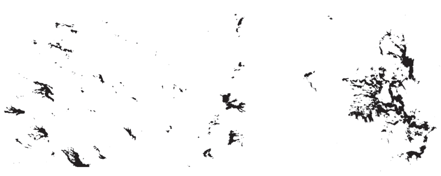
Figure 14. Morphologies of linear (left) and feathery (right) shrinkage porosity.
