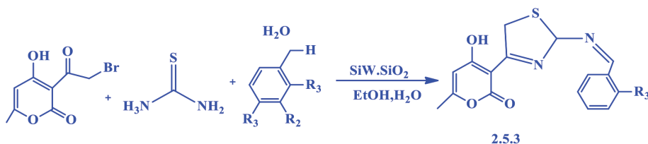
Figure 9. Synthesis of thiazole derivatives using silica.
