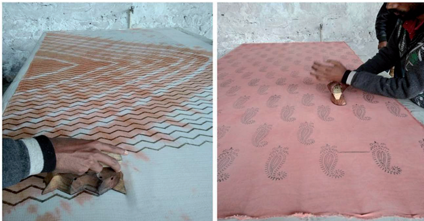
Figure 17. Printing by wooden blocks.
