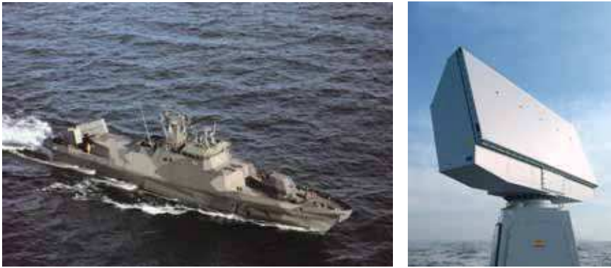
Fig. 21. TRS-3D on the Finnish guided missile boat "Hamina" (Photo courtesy of EADS)
