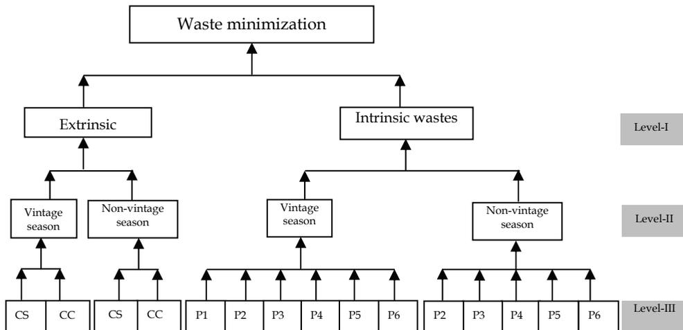
CS: Cleaning and sanitation; CC: Chemical consumption; P1: Crushing and destemming processes; P2: Transfer processes and operations; P3: Filtration, P4: Pressing; P5: Fermentation; P6: Bottling and packaging.
