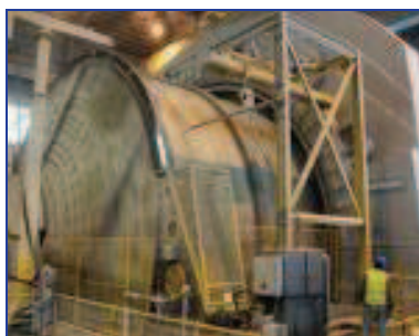
Fig. 1. Typical semi-autogenous (SAG) mills
