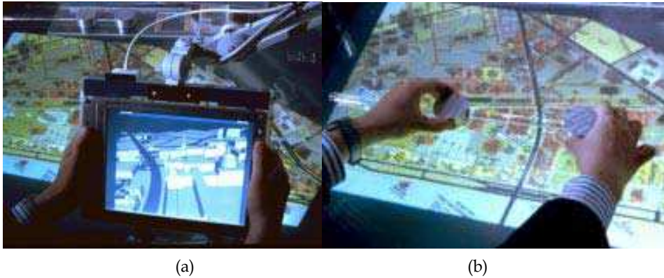
Fig. 4. (a). Active lens in tangible Geospace (b). Rotation constraint instrument (Ishii & Ullmer, 2006)
