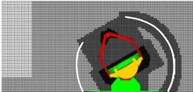
Fig. 7. Voxel distribution on a plane cutting through the telescope configuration ( $\phi = 30^\circ$  and  $\varphi = 0^\circ$ ). The enclosure cross-section is displayed in white (Mamou *et al.*, 2008)
