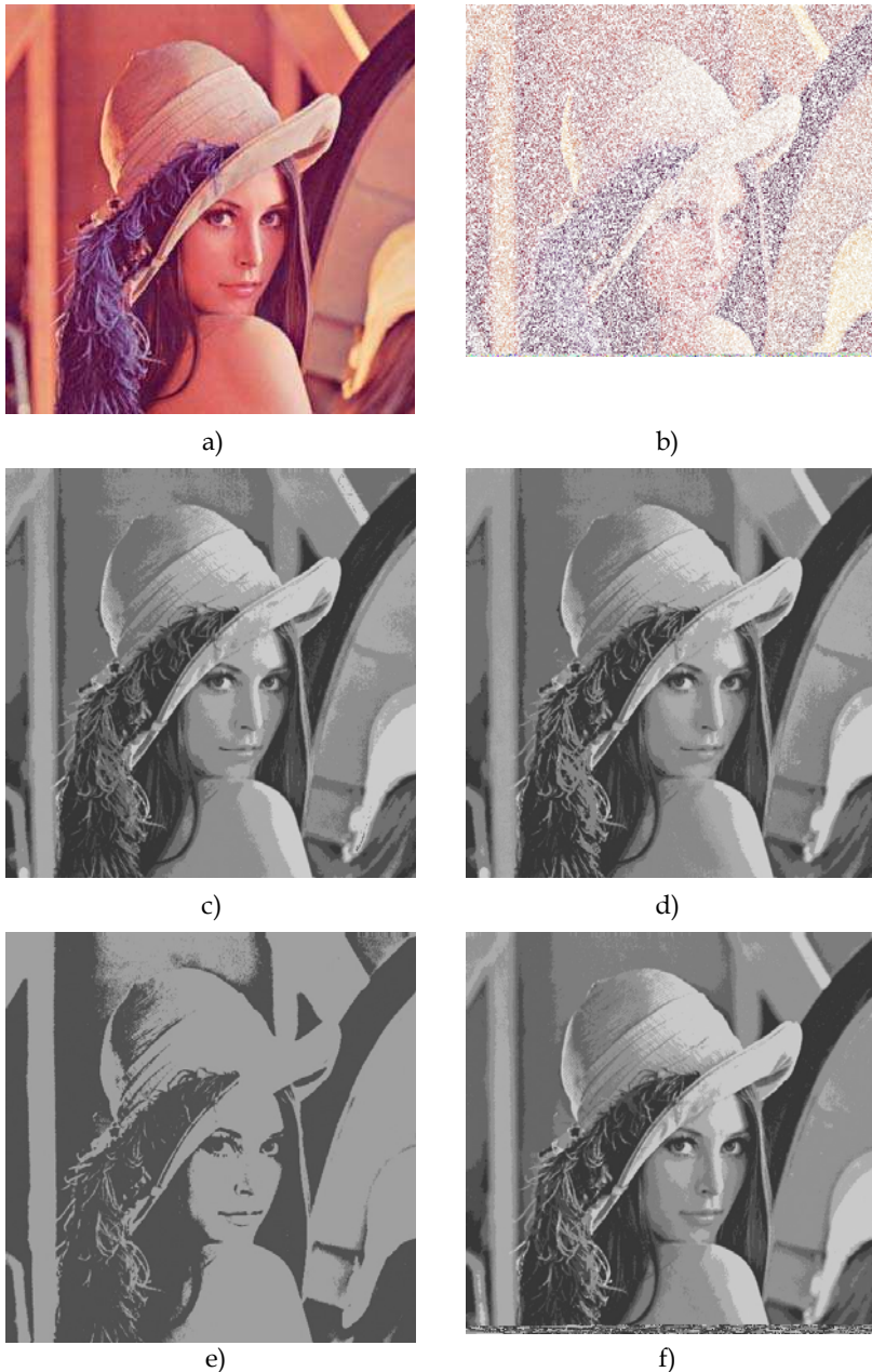
Fig. 10. The Lenna image processing: a) Original image; b) Training set (30% of the original image); c) The 1 st epoch of self-learning fuzzy spiking neural network learning; d) The 3 rd epoch of self-learning fuzzy spiking neural network learning; e) The 3 rd epoch of fuzzy c-means learning; f) The 30 th epoch of fuzzy c-means learning
