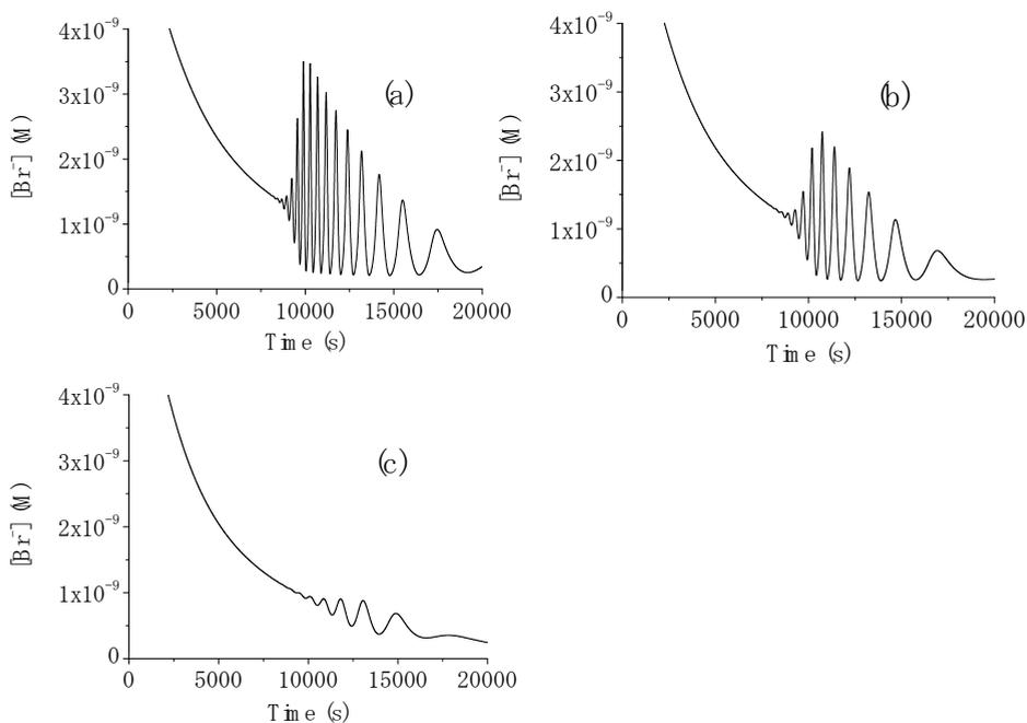
Fig. 13. Numerical simulations of the present model K1 - K14 at different initial concentrations of bromate: (a) 0.08 M, (b) 0.09 M, and (c) 0.1M. Other reaction conditions are  $[HAr(OH)_2] = 0.057$  M,  $[H_2SO_4] = 1.4$  M, and  $[Br^-] = 1.0 \times 10^{-10}$  M.
