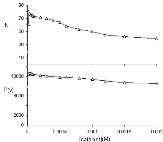
Fig. 7. Dependence of the number of oscillations (N) and induction period (IP) on the concentration of ferriin. Other reaction conditions are:  $[\text{H}_2\text{SO}_4] = 1.30 \text{ M}$ ,  $[\text{BrO}_3^-] = 0.078 \text{ M}$ , and  $[\text{pyrocatechol}] = 0.043 \text{ M}$ .
