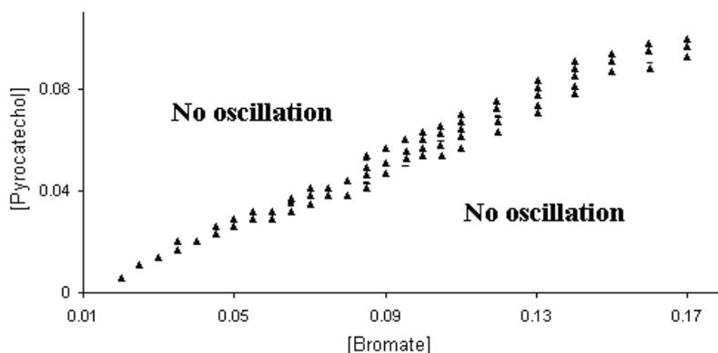
Fig. 4. Phase diagram of the bromate-pyrocatechol reaction in the pyrocatechol - bromate concentration plane. ( $\blacktriangle$ ) denotes where the system exhibits transient oscillations. Sulfuric acid concentration was fixed at 1.4 M.
