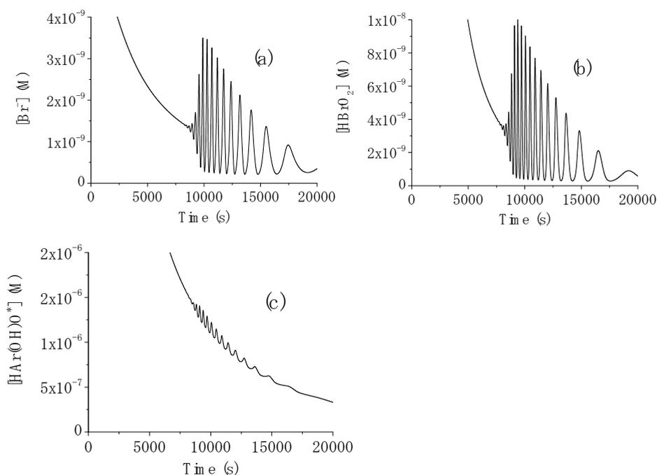
Fig. 12. Numerical simulations of oscillations in (a)  $Br^-$  (b)  $HBrO_2$ , and (c) pyrocatechol radical,  $HAr(OH)O^*$  obtained from the present model K1 - K14 by using the rate constants listed in Table 1. The initial concentrations were  $[BrO_3^-]=0.08$  M,  $[HAr(OH)_2]=0.057$  M,  $[H_2SO_4]=1.4$  M, and  $[Br^-]=1.0 \times 10^{-10}$  M; the other initial concentrations were zero.
