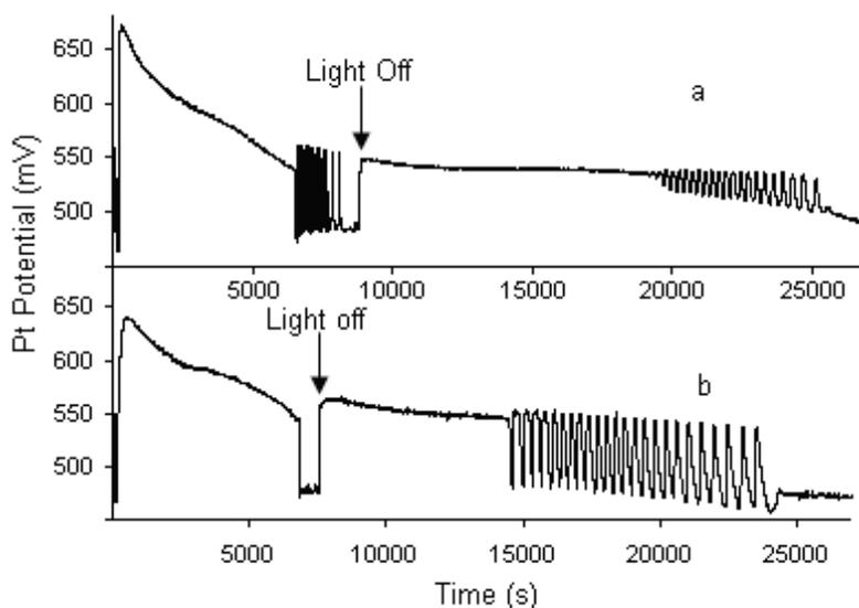
Fig. 11. Light effect on the bromate - pyrocatechol - ferroin reaction (a) and (b) light illuminating from the beginning with intensity equal to  $70 \text{ mW/cm}^2$ , under conditions  $[\text{NaBrO}_3] = 0.10 \text{ M}$ ,  $[\text{H}_2\text{SO}_4] = 1.40 \text{ M}$ ,  $[\text{H}_2\text{Q}] = 0.057 \text{ M}$ , (a)  $[\text{Ferroin}] = 5.0 \times 10^{-4} \text{ M}$ , and (b)  $[\text{Ferroin}] = 1.0 \times 10^{-3} \text{ M}$ .
