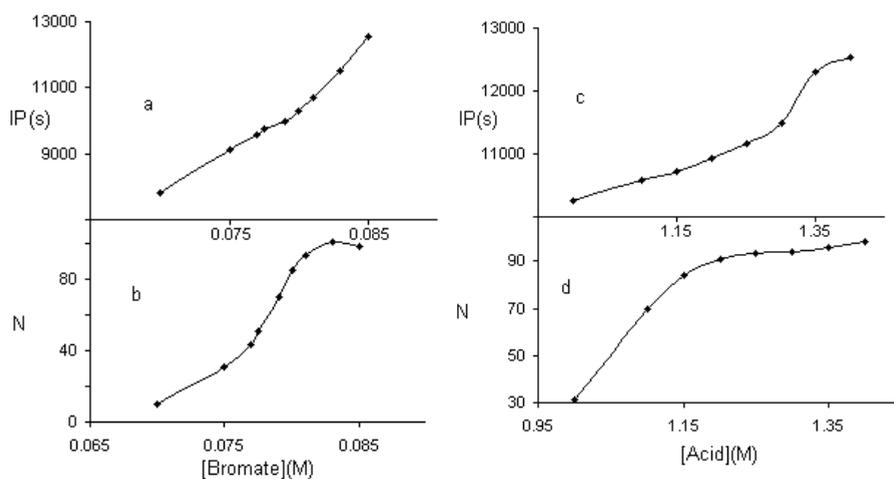
Fig. 8. Dependence of the number of oscillations (N) and induction time (IP) of the ferriin-catalyzed system on the concentration of bromate and sulfuric acid. Other reaction conditions are:  $[\text{H}_2\text{Q}] = 0.044 \text{ M}$ ,  $[\text{ferriin}] = 1.0 \times 10^{-4} \text{ M}$ , and (a & b)  $[\text{H}_2\text{SO}_4] = 1.40 \text{ M}$ ; (c&d)  $[\text{NaBrO}_3] = 0.085 \text{ M}$ .
