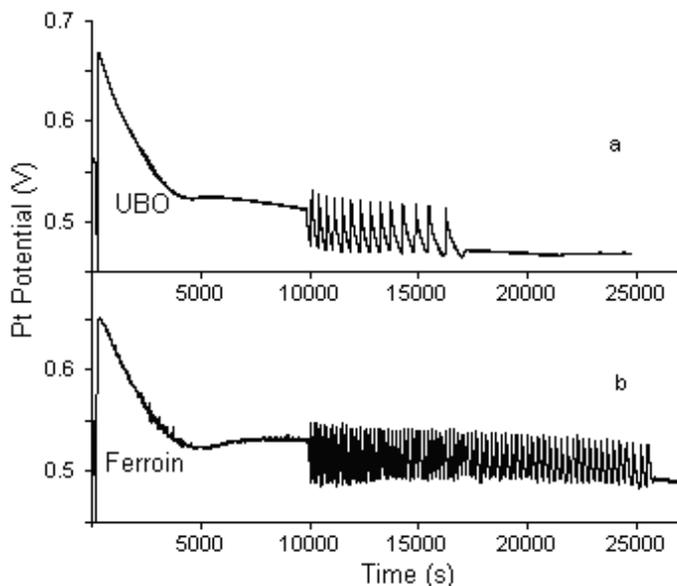
Fig. 6. Time series of the (a) uncatalyzed, and (b) ferroin-catalyzed bromate-pyrocatechol reaction. Other reaction conditions are:  $[\text{H}_2\text{SO}_4] = 1.30 \text{ M}$ ,  $[\text{H}_2\text{Q}] = 0.043 \text{ M}$  and  $[\text{BrO}_3^-] = 0.078 \text{ M}$ . The concentration of ferroin is equal to  $1.0 \times 10^{-4} \text{ M}$  in (b).
