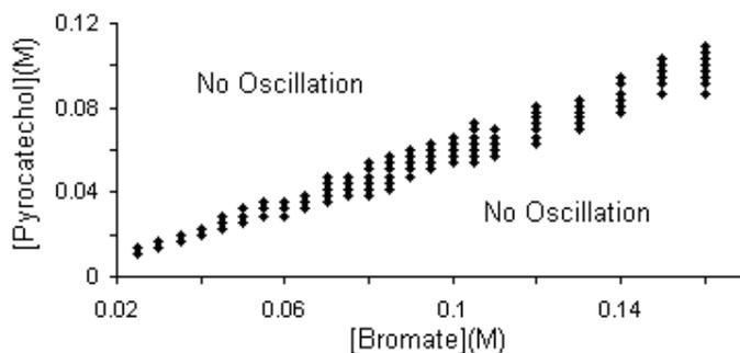
Fig. 9. Phase diagram of the ferriin-catalyzed reaction in the bromate-pyrocatechol concentration plane. ( $\blacklozenge$ ) denotes where the system exhibits simple periodic oscillations. The concentration of ferriin is  $1.0 \times 10^{-4}$  M.
