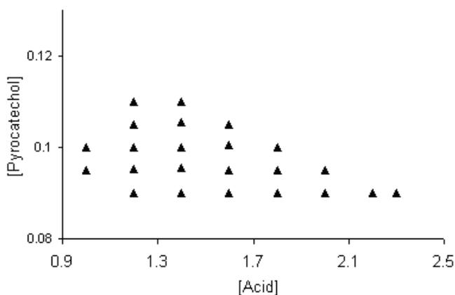
Fig. 5. Phase diagram of the bromate-pyrocatechol reaction in the bromate -  $\text{H}_2\text{SO}_4$  concentration plane. ( $\blacktriangle$ ) denotes the conditions under which the system exhibits oscillations. The concentration of pyrocatechol is 0.057 M.
