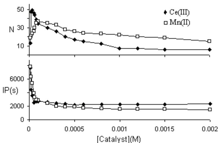
Fig. 10. Dependence of the number of oscillations ( $N$ ) and induction time ( $IP$ ) on the initial concentrations of cerium and manganese. Other reaction conditions are  $[\text{H}_2\text{SO}_4] = 1.3 \text{ M}$ ,  $[\text{NaBrO}_3] = 0.078 \text{ M}$ , and  $[\text{H}_2\text{Q}] = 0.043 \text{ M}$ .
