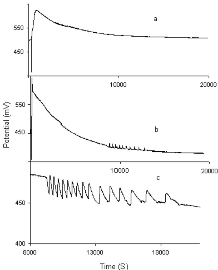
Fig. 1. Time series of the pyrocatechol - bromate reaction at different initial concentrations of bromate: (a) 0.085 M, (b) 0.093 M and (c) 0.095M. Other reaction conditions are  $[H_2Q] = 0.057$  M, and  $[H_2SO_4] = 1.4$  M.
