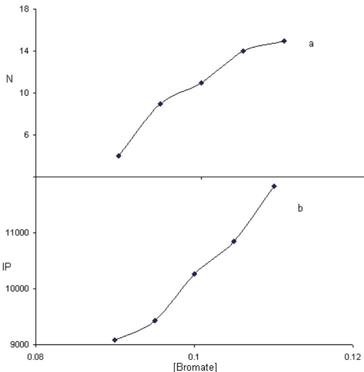
Fig. 2. Dependence of the number of oscillations ( $N$ ) and induction period ( $IP$ ) on the initial concentration of bromate. Other reaction conditions are  $[H_2Q] = 0.057$  M and  $[H_2SO_4] = 1.2$  M.
