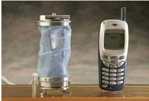
Figure 1. The SpineAssist miniature robot
