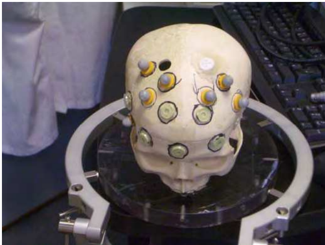
Figure 9 a. A photograph of the human head phantom with surface targets (buttons) and robotic fiducials (reflective balls)
