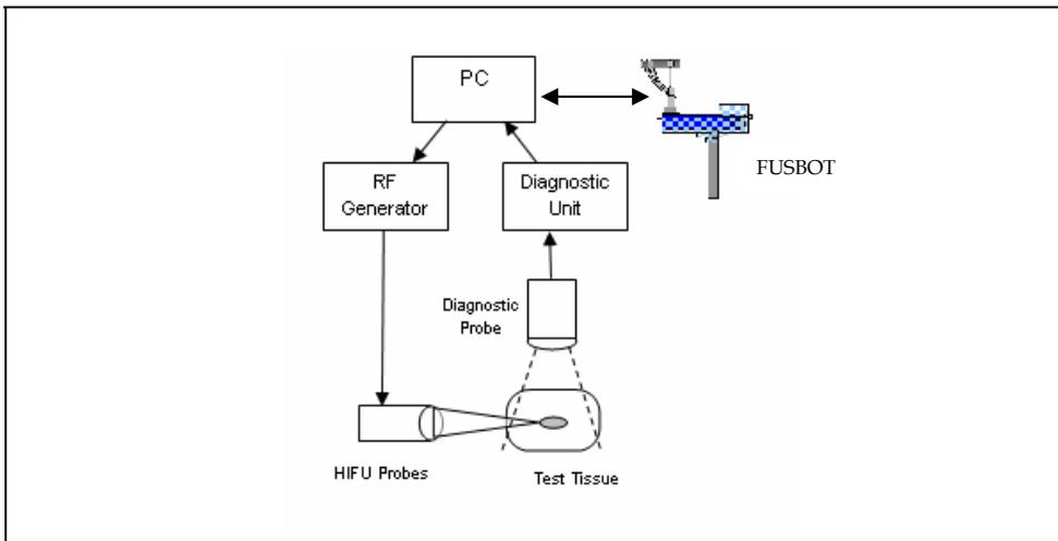
Figure 1. System schematic diagram - experimental set-up
