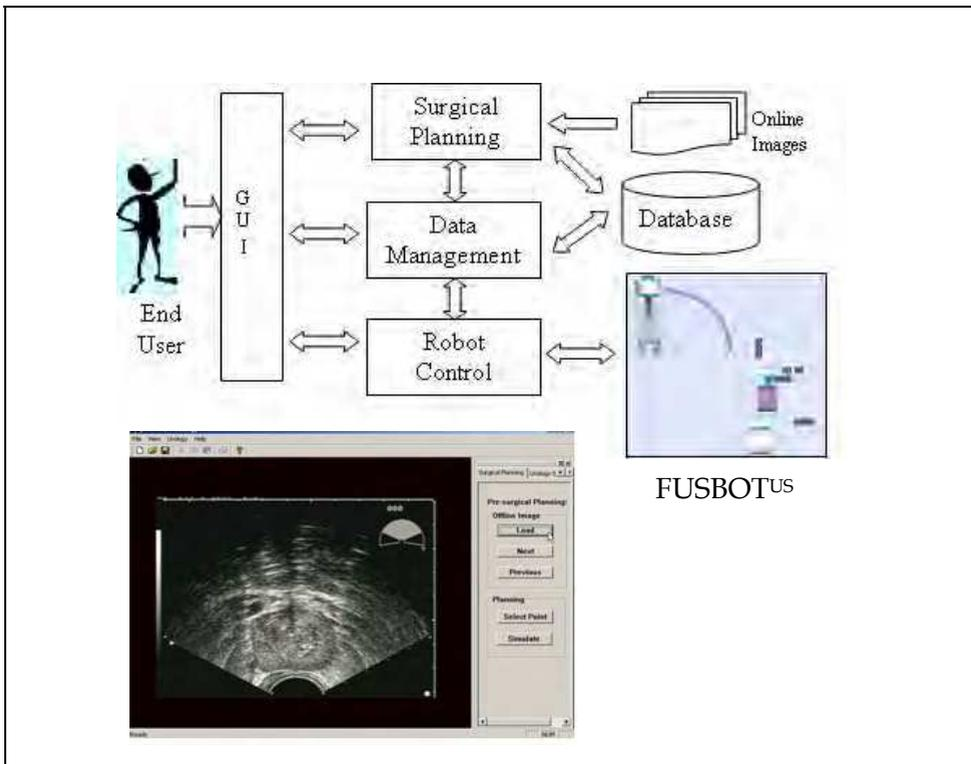
Figure 3. FUSBOT<sup>US</sup>: Urological Surgery System - Software structure of control module; Graphical User Interface
