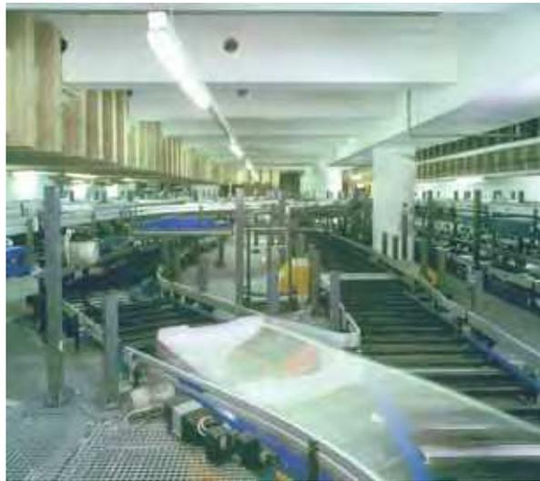
Figure 3. Snapshot into a BHS with a moving tote in the foreground
