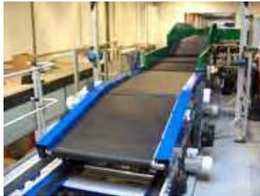
Figure 6. A toploader, where bags arrive on a traditional conveyor belt
