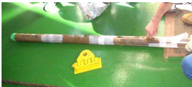
Fig. 17. Mud sample obtained from the sea floor in the Mariana trench (2m-core sampler)
