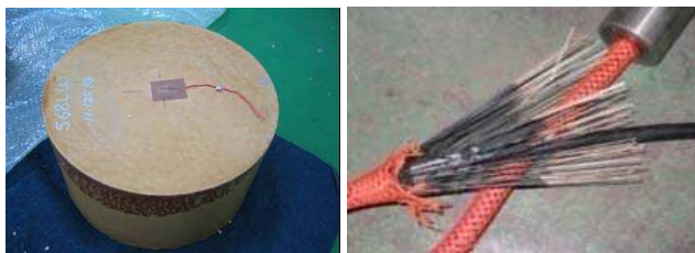
Fig. 1. A prototype of the full ocean depth buoyancy material (left) and the secondary cable made from para-aramid fiber (right).
