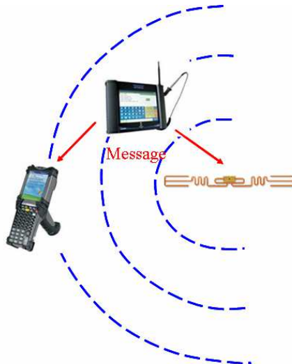
Fig. 5. Eavesdropping on reader-tag communication
