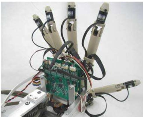
Fig. 9. Developed circuits installed in HIRO II+.
