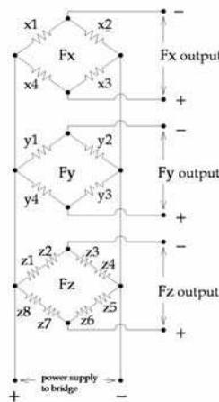
Fig. 13 Bridge circuit.
