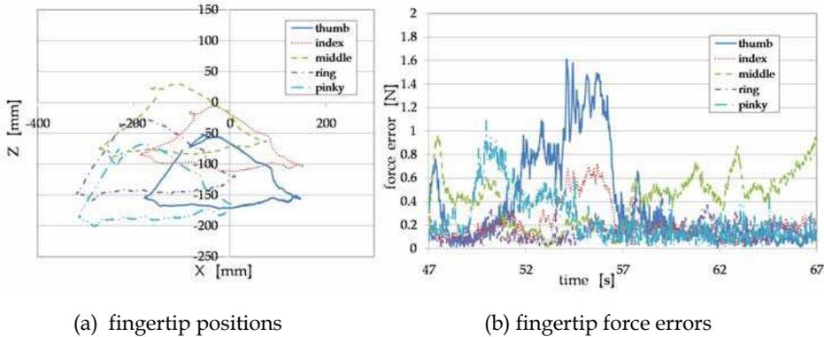
Fig. 22. Responses of HIRO II<sup>+</sup> with former force sensor in constraint space.
