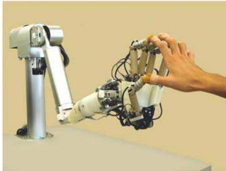
Fig. 1. Five-fingered Haptic Interface Robot: HIRO II<sup>+</sup>.
