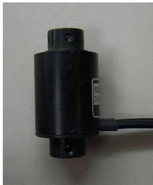
Fig. 10 Three-axis force sensor.
