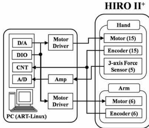
Fig. 5. Control system of HIRO II<sup>+</sup>.
