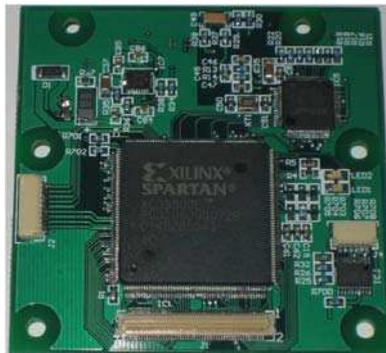
Fig. 7. Interface FPGA circuit.
