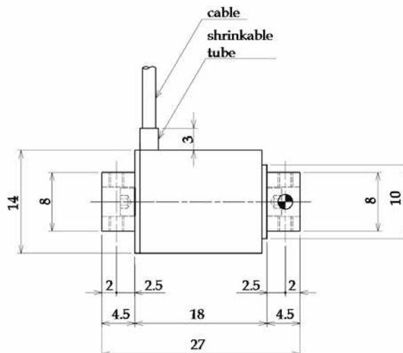
Fig. 11 The dimensional drawing of the force sensor.
