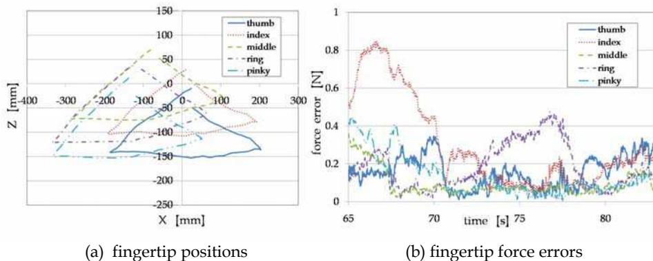
Fig. 21. Responses of HIRO II<sup>+</sup> with developed force sensor in constraint space.
