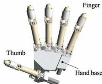
Fig. 3. Haptic hand design.
