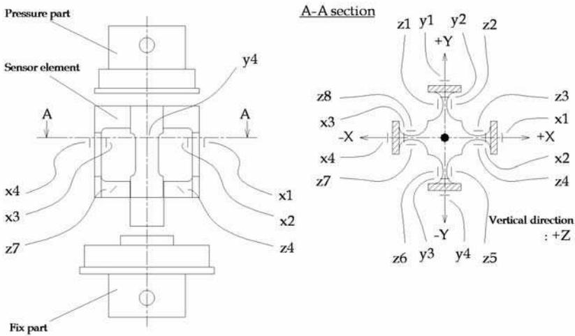
Fig. 12 Force sensor structure.
