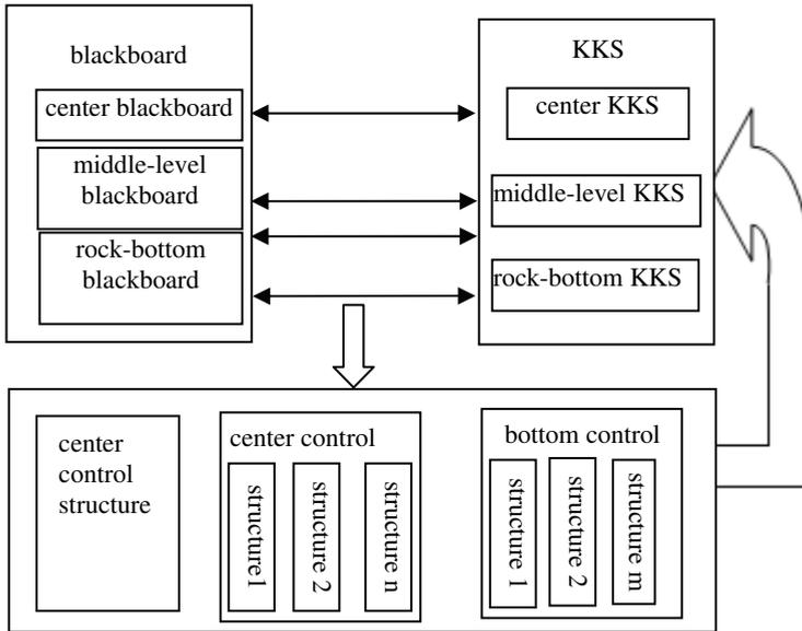
Fig. 3.1 Multilevel blackboard model of packing line system
