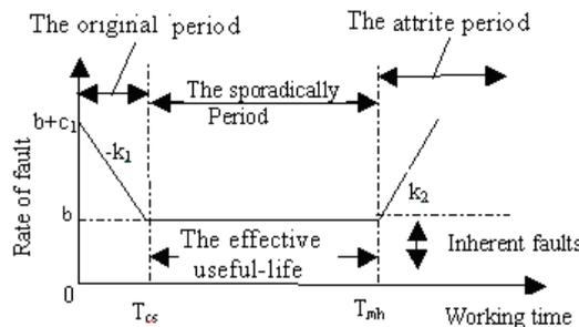
Fig. 2.3 Simplified graph of equipment fault ratio
