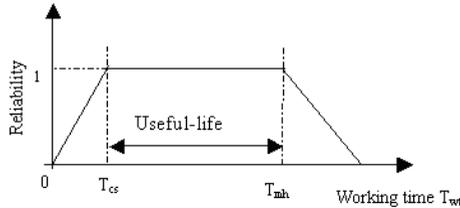
Fig. 2.4 The relationship between reliability and working hours
