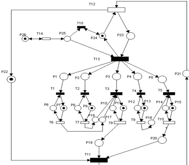
Fig. 3.2 Petri Net coordination model of multi-agent system
