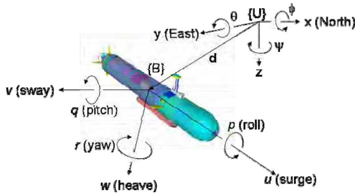
Fig. 7. Frames definition for an UV.
