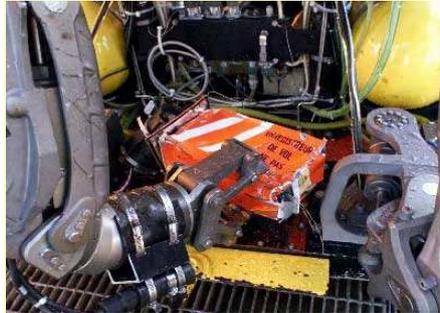
Fig. 4. black-box recovery using ROV, form U.S. Dept. of Defence.
