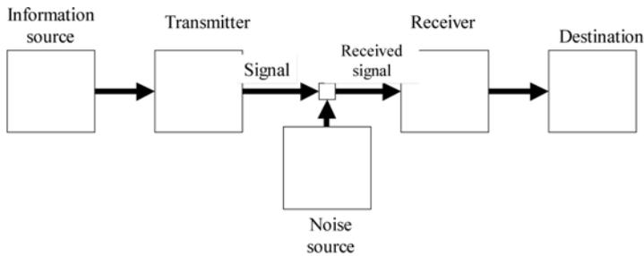
Fig. 1. Schematic diagram of general communication system
