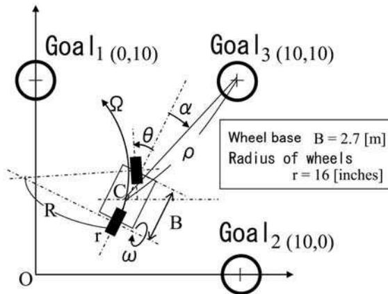
Fig. 8. State variables and parameters in task environment
